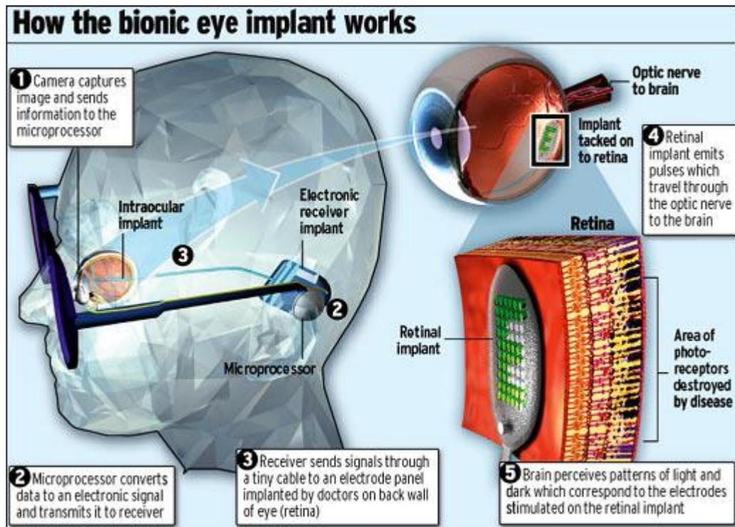
Fig 5.3. Working of bionic eye<sup>[7]</sup>
