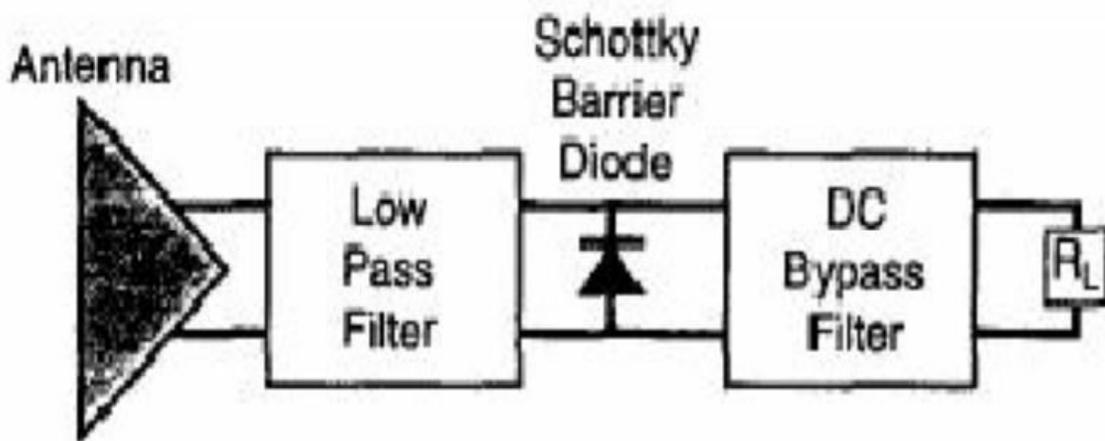
**Fig.5.1 Block diagram of Rectenna.**
