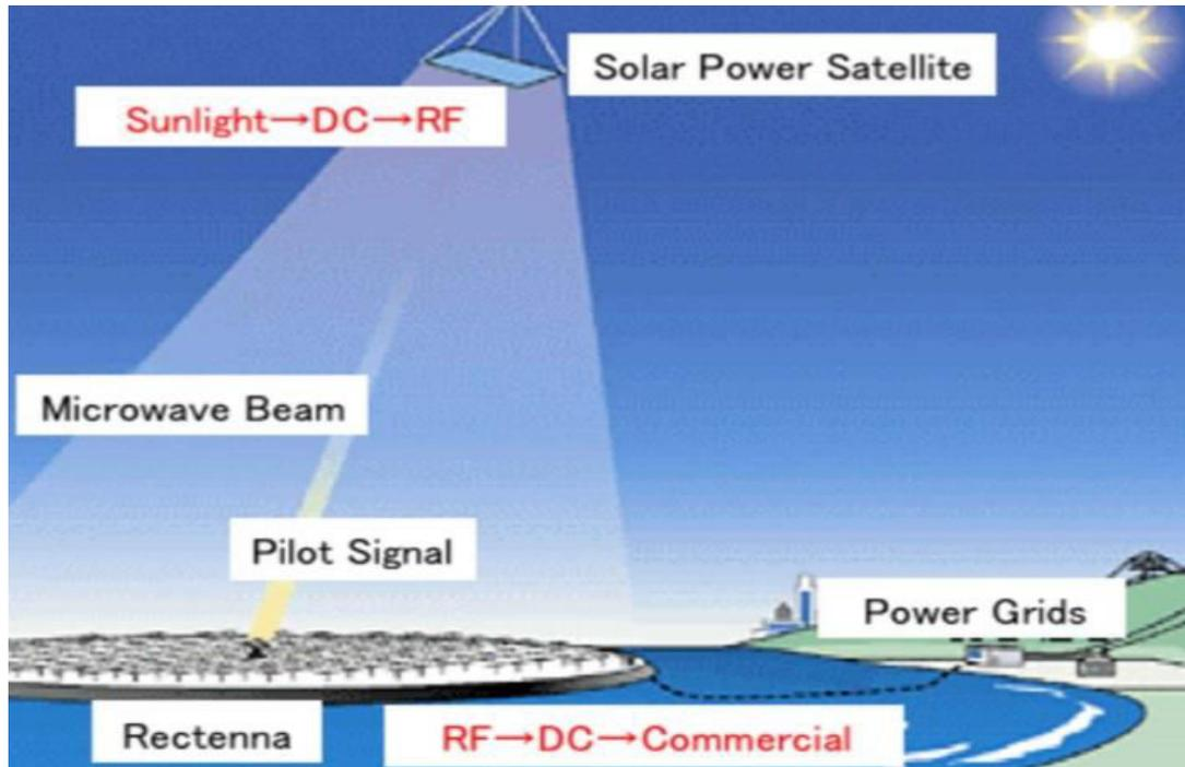
**Fig.1.1 Configuration of the SPS System.**
