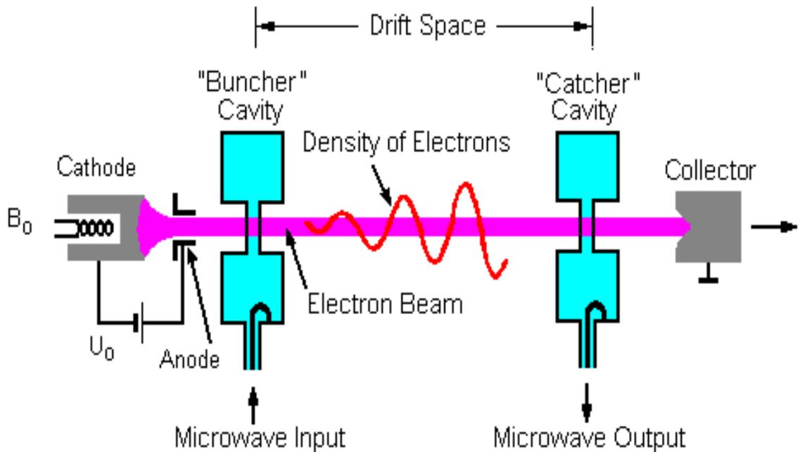
**Fig.4.1 Klystron amplifier schematic diagram.**
