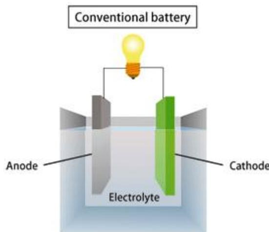
*Figure 1.1 Typical battery structure [1]*
