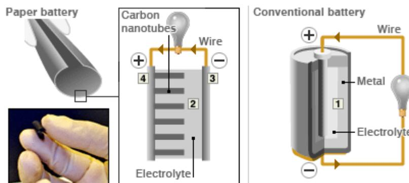
*Figure 4.1 Paper battery working [4]*
