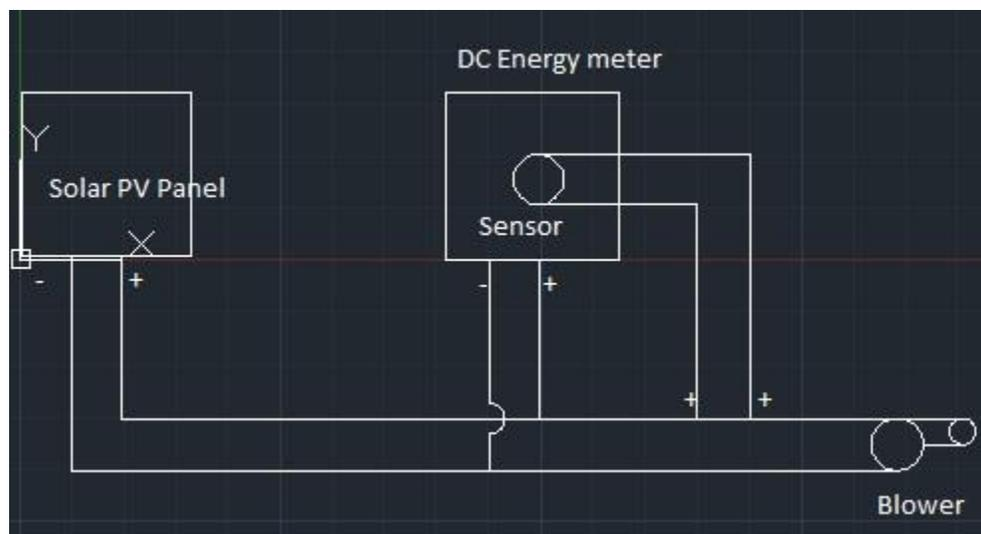
Figure 3.3: Schematic diagram Of Solar Electric circuit
