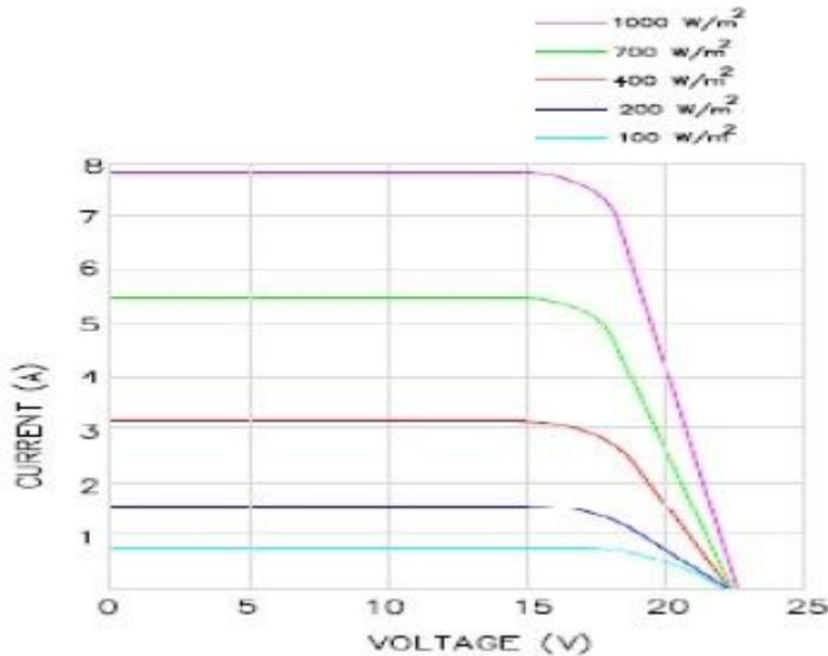
**Figure 3.1: Solar Panel I vs. V**
