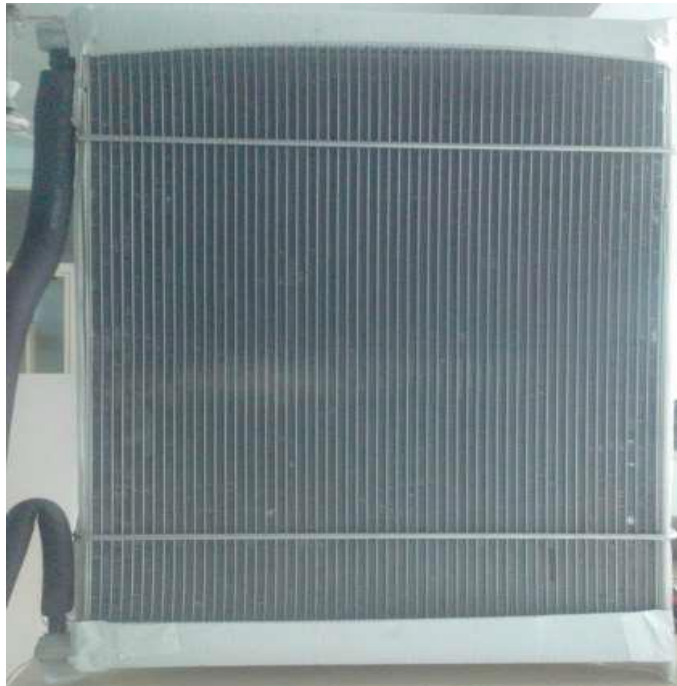
Fig.3.2: MCHX as evaporator
