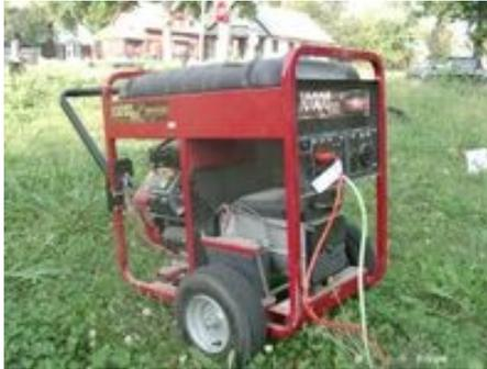
**Fig 3.1** Portable generator side view showing gasoline engine.
